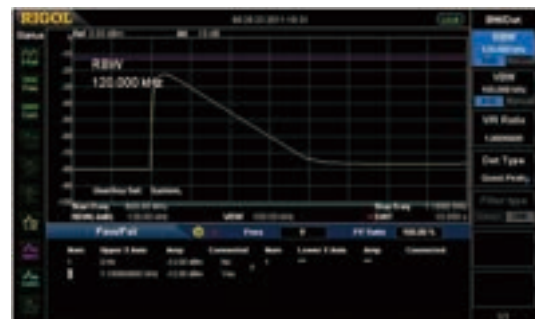
EMI kit (EMI filter & Quasi-peak & Pass/Fail)
