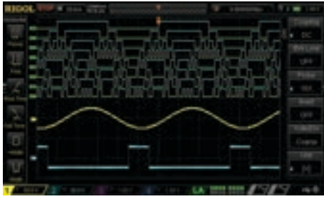
4 analog channels and 16 digital channels (supported only when the DS1000Z Plus is upgraded with the MSO upgrade option)
