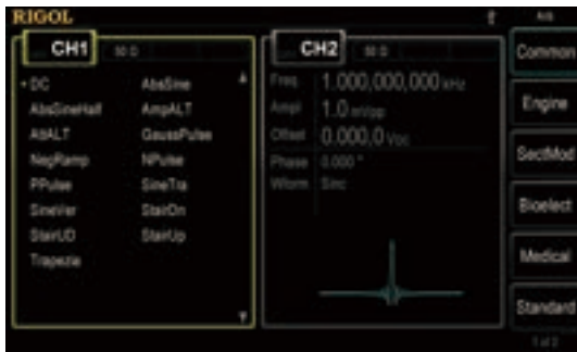
Arbitrary waveform editing (std.) and 150 built-in arbitrary waveforms
