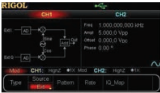
Support internal and external IQ modulation (std.)
