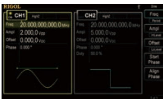
Dual channels with identical functions and phase adjustable between channels
