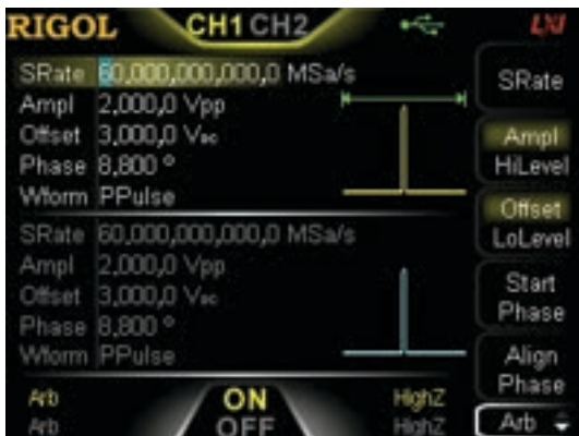
Arbitrary waveform function with innovative SiFi technology
