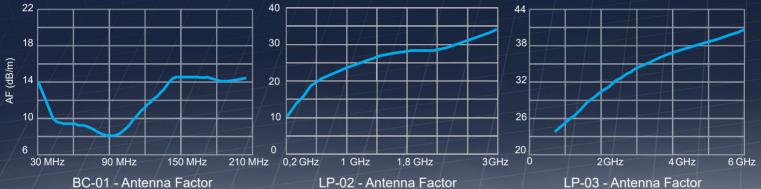
AS-03 antenna set 30 MHz to 6 GHz with individual calibration reports. AS-03/TC antenna set 30 MHz to 6 GHz with typical calibration reports. Includes: BC-01 biconical antenna, LP-02 log-periodic antenna, LP-03 log-periodic antenna, TR01 wooden column tripod, antenna mounting adapter to change polarization, 5 meter/6 GHz/N(m)-N(m) RF cable, N(f)-N(f) adapter, soft carrying case, user's manual, calibration reports'
