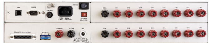
MODEL SC6540 GGM* 16 Channel High Current Multiplexer
