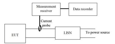
Conducted emission, differential mode, measurement setup
