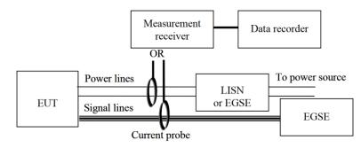
Conducted emission, common mode, measurement setup \*) EGSE: electrical ground support equipment
