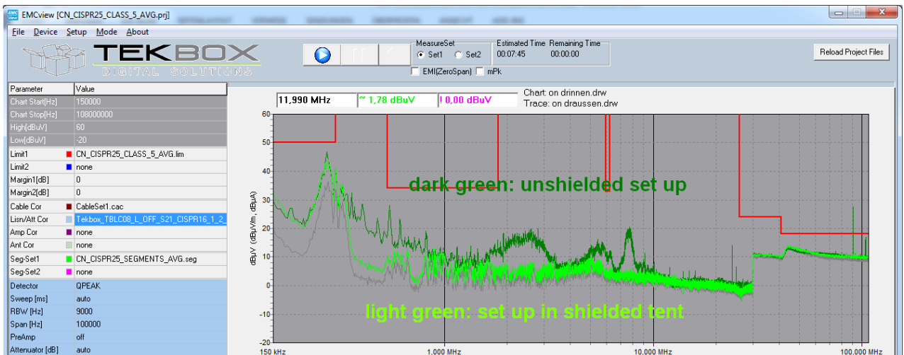
Picture 6: CISPR 25 conducted noise measurement; DUT powered
