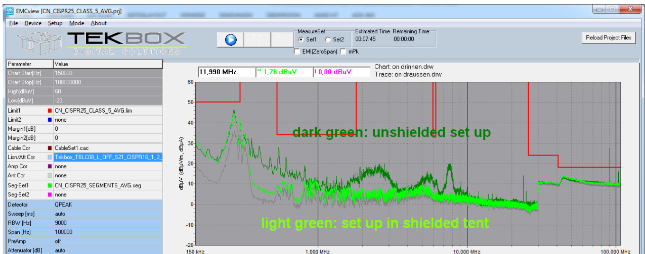
Picture 6: CISPR 25 conducted noise measurement; DUT powered
