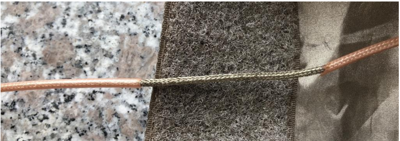
Picture 11: feed through using coaxial cable with stripped jacket
