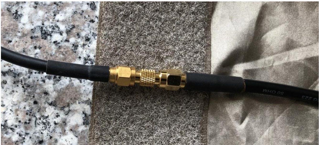
Picture 9: feed through using coaxial adapter
