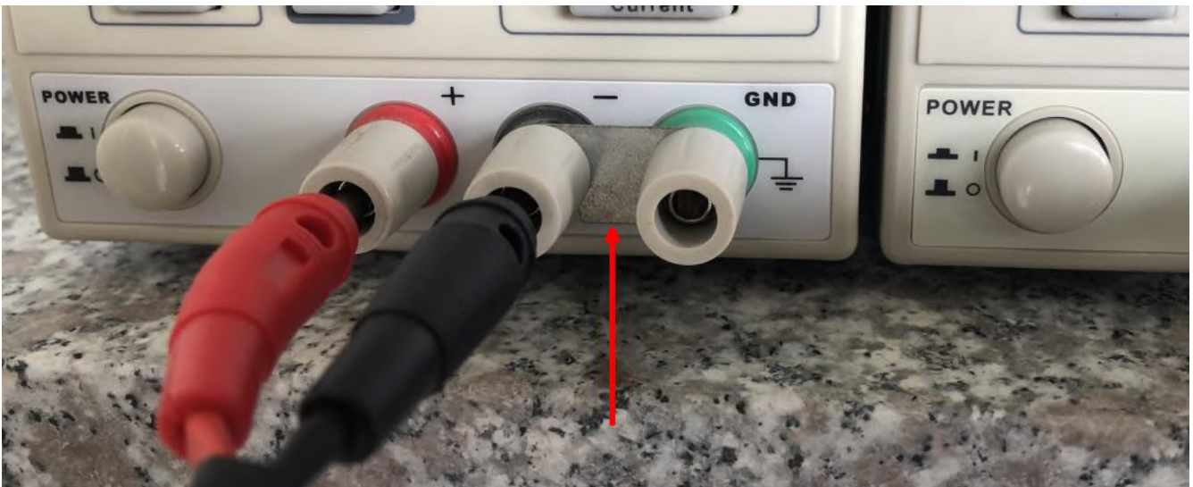
Picture 16: DUT supply at power supply side; connect power supply ground with housing earth
