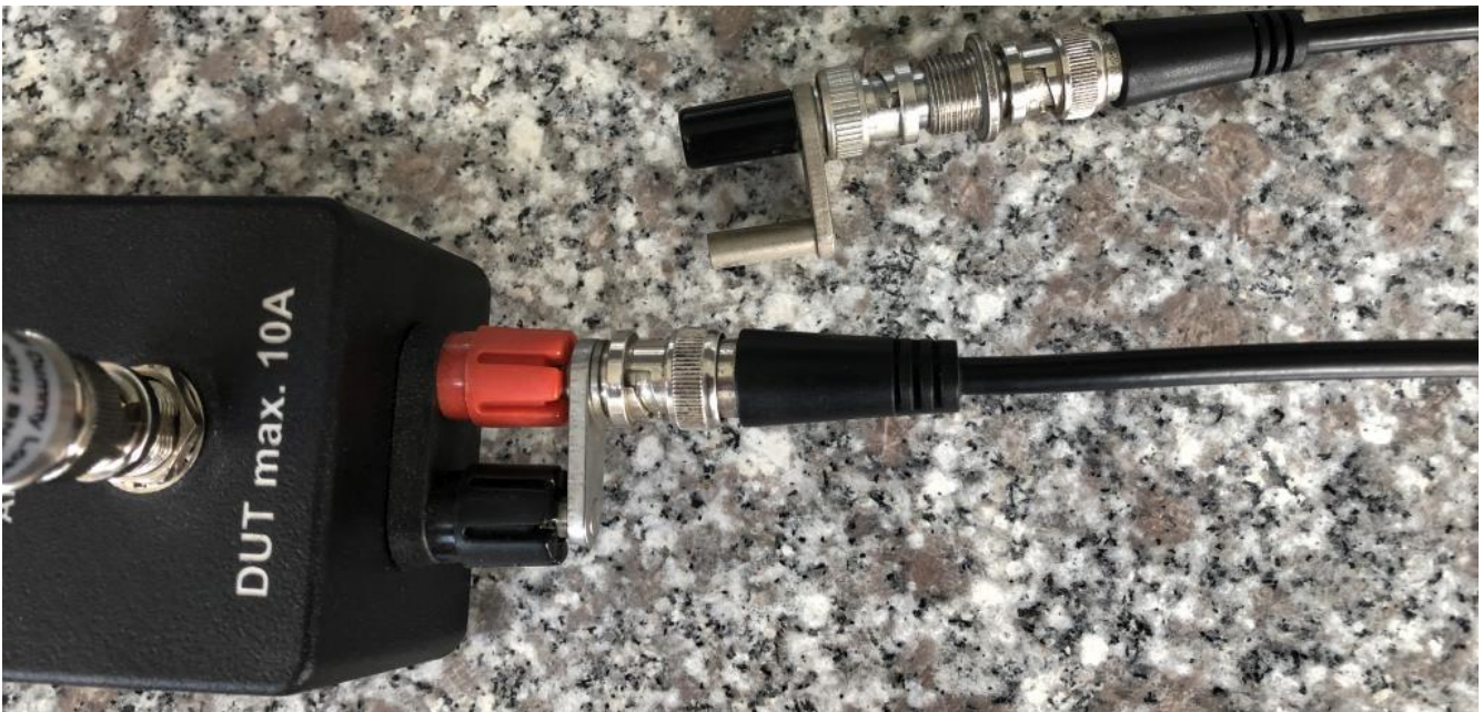
Picture 18: using banana to BNC adapters and a BNC cable as shielded supply line
