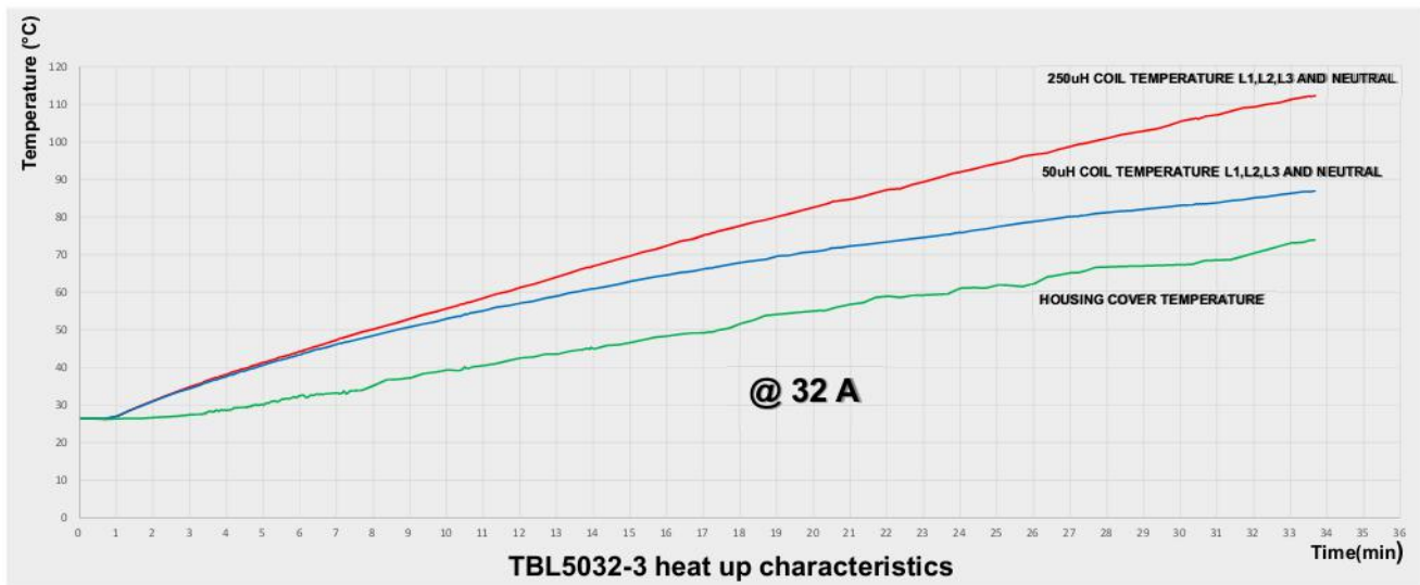
Figure 103: Coil and housing temperature at 32 A DUT current @ 22 °C ambient temperature
