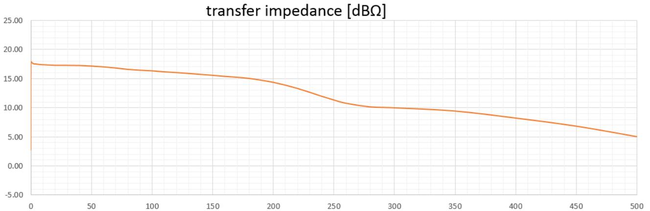
Figure1: Transfer impedance: 10 kHz to 500 MHz, linear
