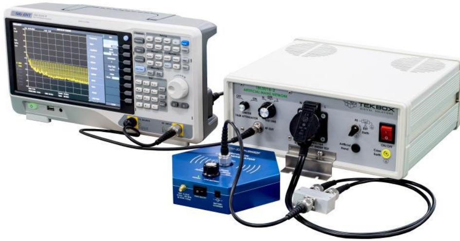
Picture 1: TBCG3-CN connected to a LISN utilizing a RF power splitter
