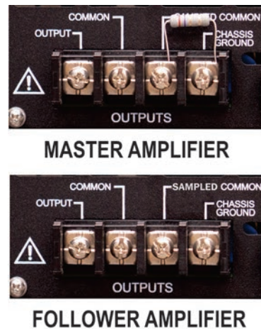
Figure 6.29 – Remove the 2.7-ohm resistor from Follower amplifiers
