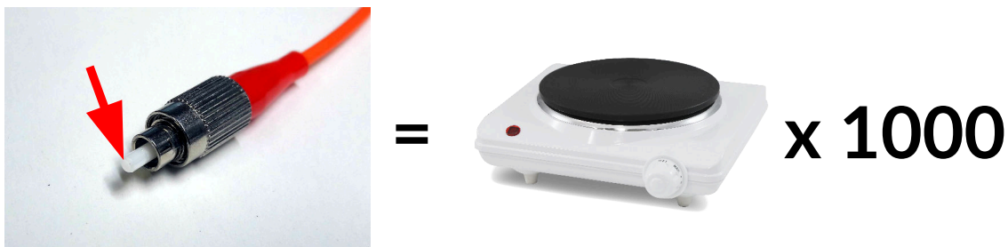
Figure 3: Power density comparison: 1 Watt fiber core vs. 1 Kilowatt hot plate
