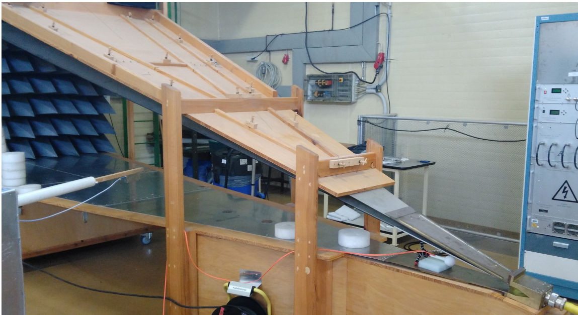
Figure 1: GTEM wave guide and pulse generator
