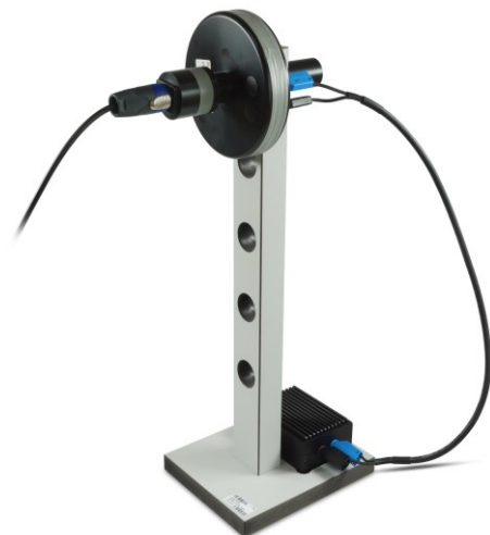
Construction radiating loop MGA RL 120
