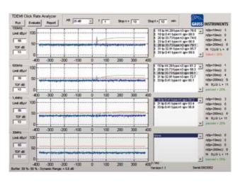
Fig. 12 - Measurement with Click Rate Analyzer according to CISPR 14.
