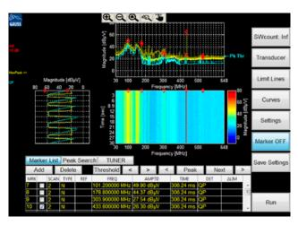
Fig. 8 – Screenshot of 645 MHz Real-time Measurement (Peak and Quasi-peak parallel).
