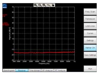
Fig. 10 – Noise floor up to 1 GHz of the TDEMI  $^\circ$  X with option ULNA-UG1G.
