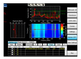
Fig. 3 – Parallel measurement of Quasi-Peak and Average with 645 MHz real-time bandwidth.
