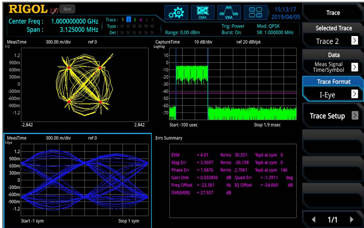
Figure 16: Digital modulation analysis at RF interface during stress situation
