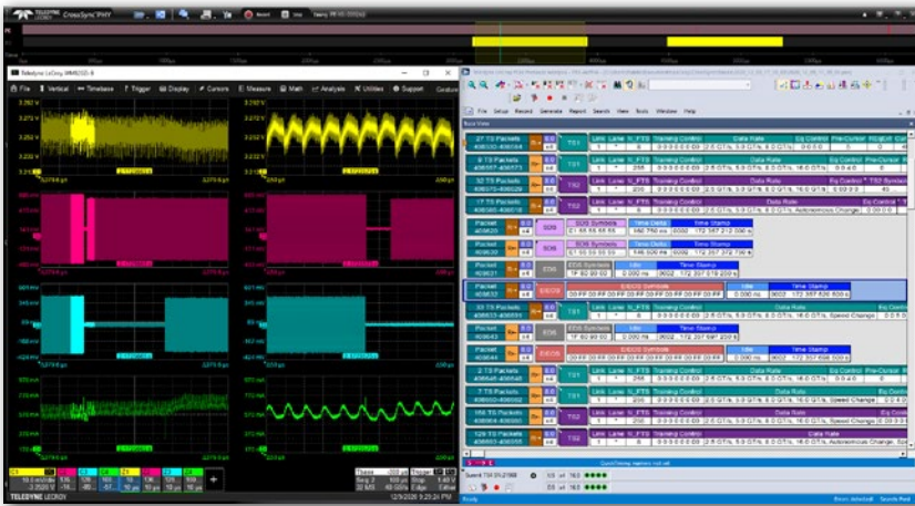
Correlated electrical and protocol views of a link speed change from 8 to 16 GT/s.
