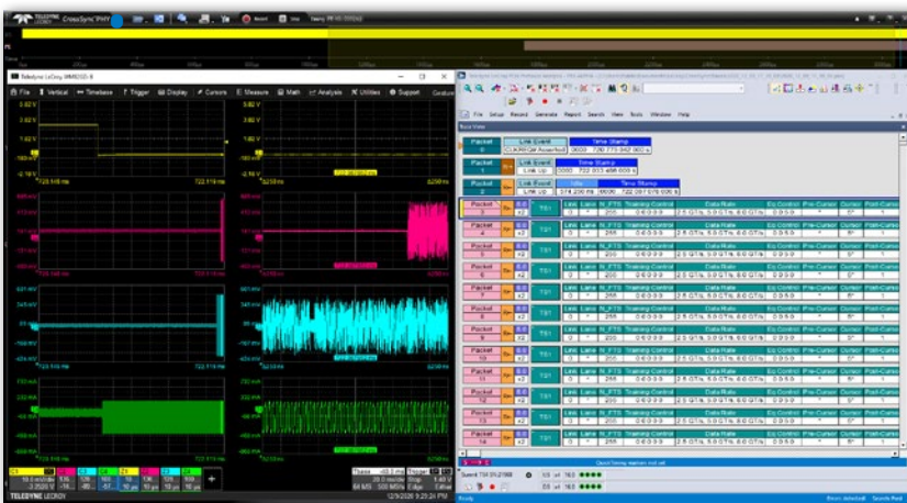
Analyzing exit from L1.2 including reference clock and CLKREQ# behavior.
