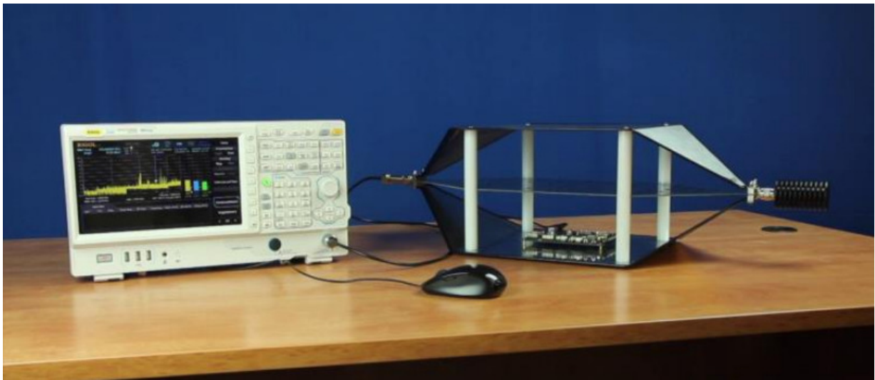
Figure 14: Repeatably radiated emission analysis with an open TEM cell
