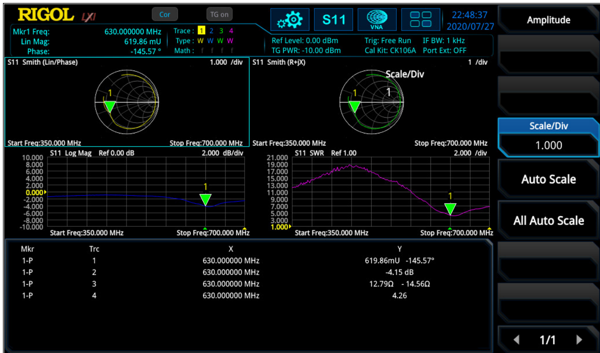
Figure 17: VNA Mode with different window of S 11 parameter like smith- and Polar Plane, logarithm. Magnitude and SWR
