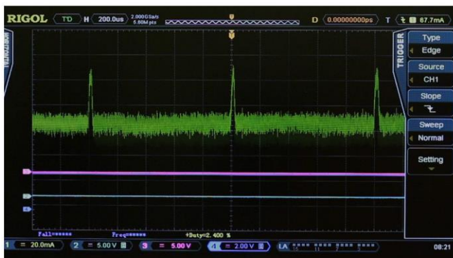
Figure 3: Pulsed current draw from battery on IoT development Platform
