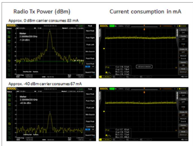
Figure 4: Current draw from Bluetooth Radio transmit test
