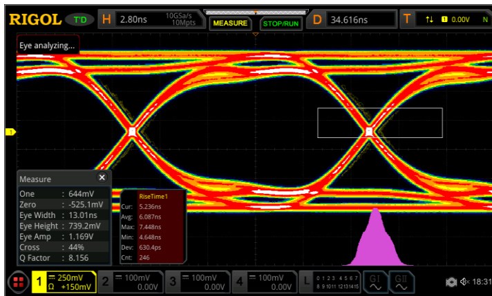
Figure 13: Eye Diagram with improved noise
