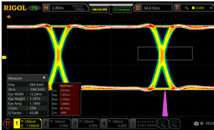
Figure 14: Eye Diagram after debugging and improvements
