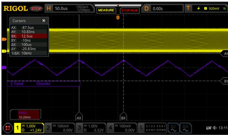
Figure 3: TIE trend graph cursor measurements
