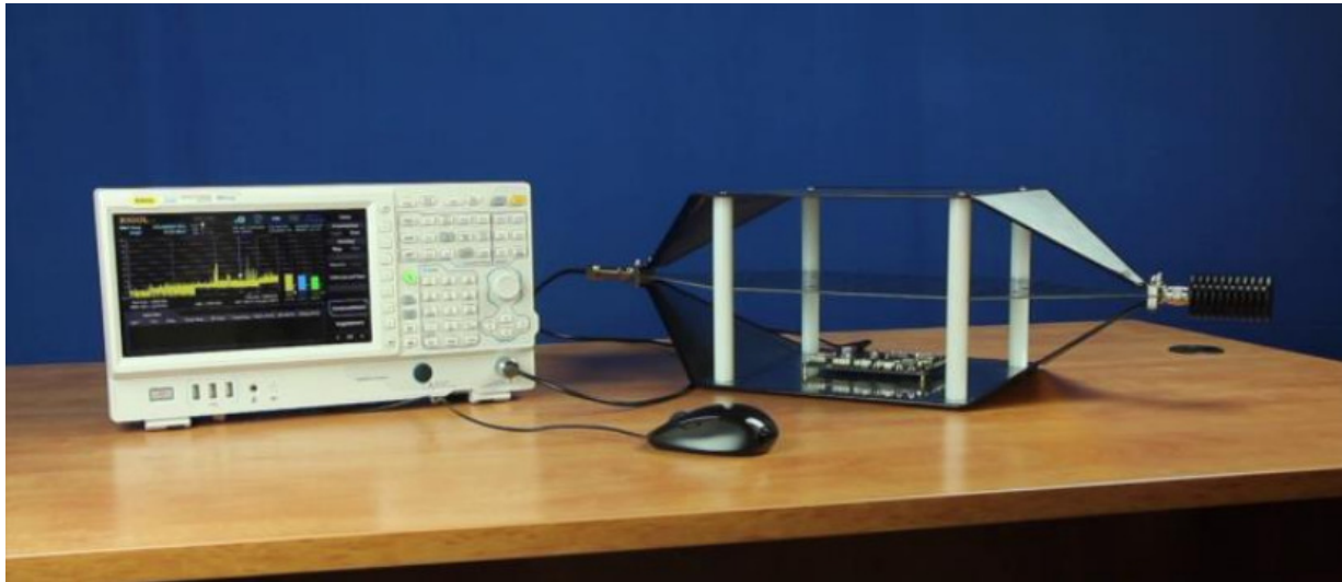
Figure 14: Repeatabile radiated emission analysis with an open TEM cell
