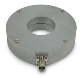
Current Monitoring probes may be used for RF current measurements with the advantage that there is no loading of the circuit, thus allowing normal operation of the DUT while the measurement is done. The CDG CMP-46 measures RF common mode currents (asymmetrical currents) of single conductors or bundles of conductors (the sum of currents considering the sign is of importance).
