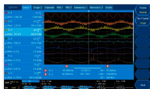
Display of sampling values of 16 signals in two scopes
