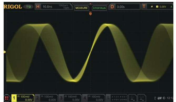
Changes of each frame of waveforms of the sweep signal can be clearly observed in the highly refreshed mode.
