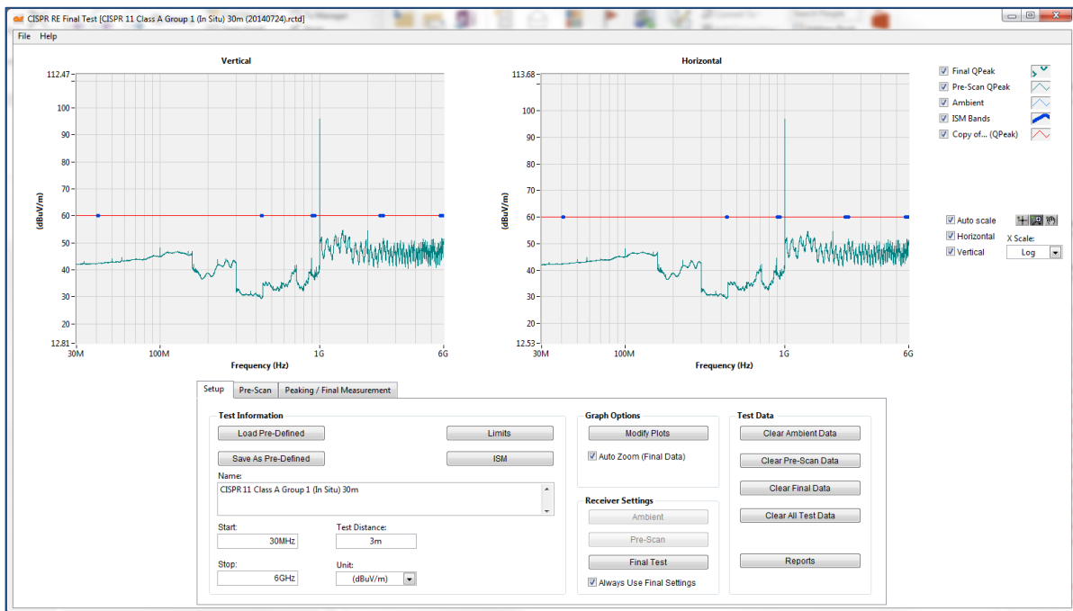
Figure 9 – CISPR Radiated Emissions
