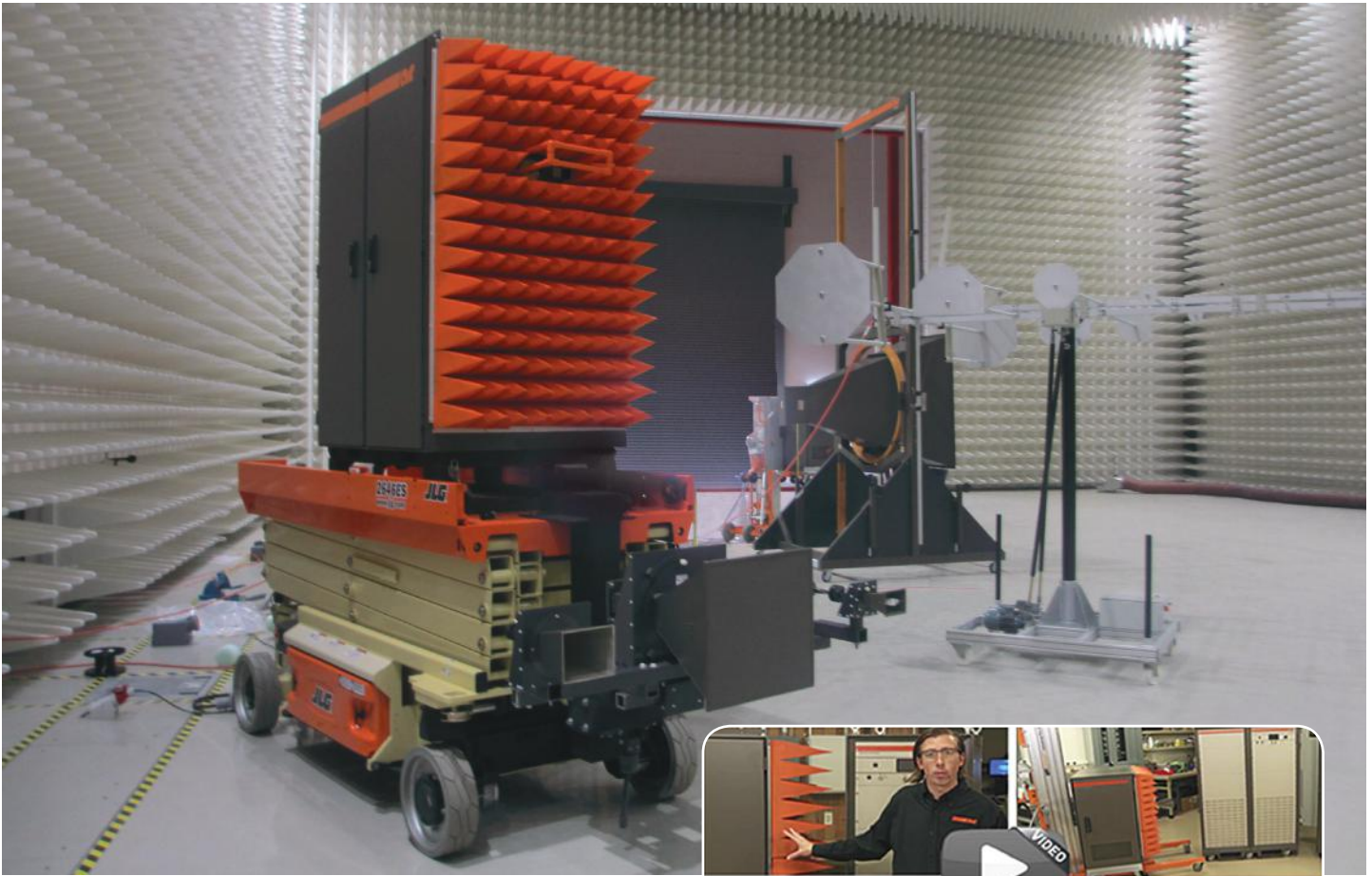
SP1053 1-18 GHz, MIL-STD-461, 200V/m, Radiated Immunity System on an electric scissor lift with a 1-6m adjustable antenna height.
