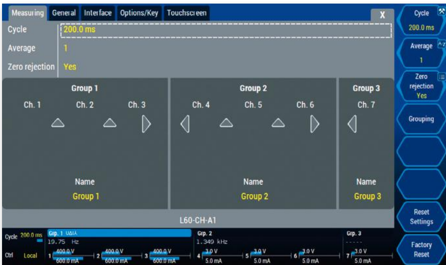
Logical grouping of channels for different points of measurement in the LMG600 configuration menu
