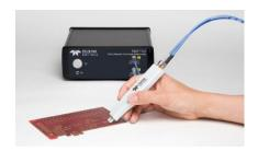
Based on the true differential design, there is no need for a physical ground connection if differential lanes are measured.
