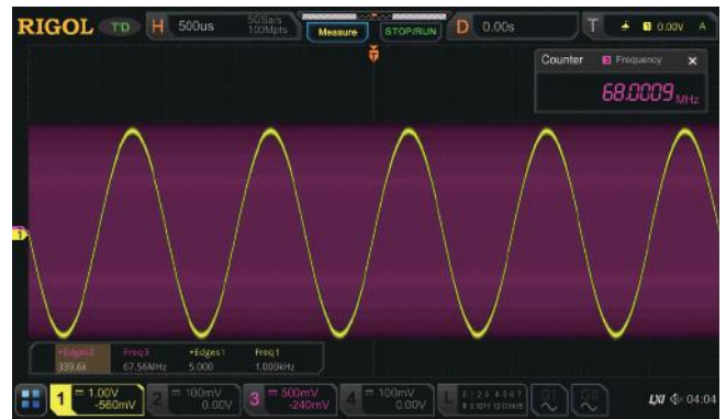
Observe and accurately measure two signals with great frequency deviations.
