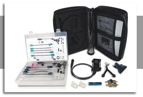
The WaveLink Differential Probe Series is a 8-13 GHz bandwidth active differential probe series with high input dynamic range, a large offset capability, and a wide variety of tips and leads available for different applications.
