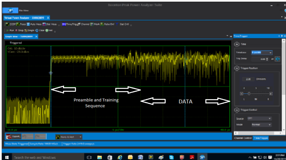
Figure 2. The beginning of a frame, including the preamble and training sequence, followed by the beginning of the OFDM signal captured with a Boonton RTP5006.
