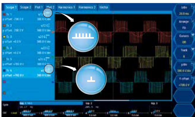
Scope display of the voltages at the converter output. The wideband values (PWM) show the PWM signal, the narrowband values (sinusoidal) are sinusoidal.
