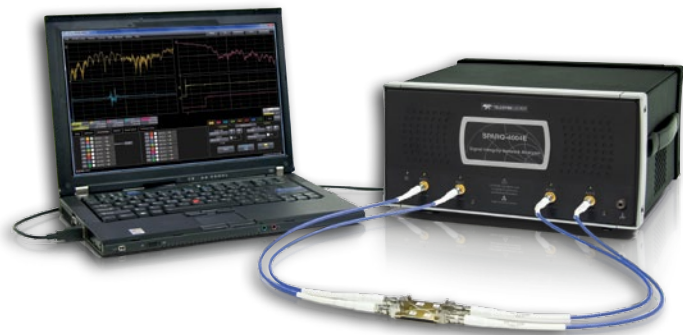
Signal Integrity Studio integrates seamlessly with the Teledyne LeCroy SPARQ, providing measurement, modeling and simulation in a single software package.
